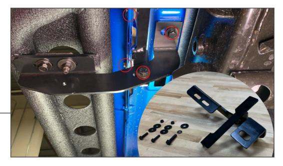
Begin at the passenger front (PF) mounting location. Loosely assemble the brackets as shown. (2) M6x1.00 25mm bolts, (4) M6 washers, (2) M6 lock nuts will secure the pinch weld bracket to the vehicle. (1)M10x1.50 30mm bolt, (2) M10 washers, (1) M10 lock nut will secure the pinch weld bracket to the rocker step bracket. (1) M8x1.25 35mm bolt, (1) lock washer, (1) flat washer will secure the rocker step bracket to the vehicle.
