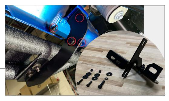
Then, at the passenger rear (PR) mounting location. Loosely assemble the brackets as shown. (2) M6x1.00 25mm bolts, (4) M6 washers, (2) M6 lock nuts will secure the pinch weld bracket to the vehicle. (1)M10x1.50 30mm bolt, (2) M10 washers, (1) M10 lock nut will secure the pinch weld bracket to the rocker step bracket. (1) M8x1.25 35mm bolt, (1) lock washer, (1) flat washer will secure the rocker step bracket to the vehicle.
