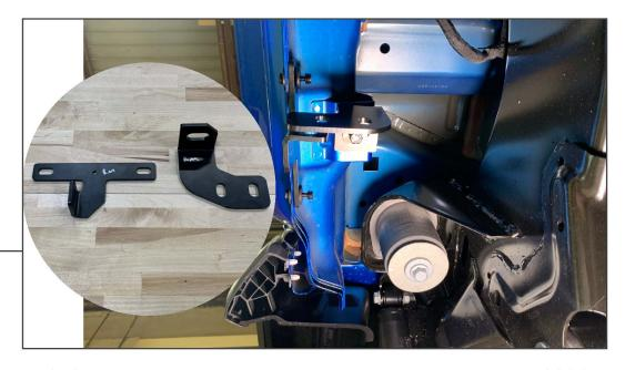
Then, passenger rear (PR) mounting location. Loosely assemble the brackets as shown. (2) (2) M6x1.00 25mm bolts, (4) M6 washers, (2) M6 lock nuts will secure the pinch weld bracket to the vehicle. (1) M8x1.25 35mm bolt, (1) lock washer, (1) flat washer will secure the rock slider bracket to the vehicle.
