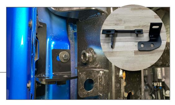
Begin at the passenger front (PF) mounting location. Loosely assemble the brackets as shown. (2) M6x1.00 25mm bolts, (4) M6 washers, (2) M6 lock nuts will secure the pinch weld bracket to the vehicle. (1) M8x1.25 35mm bolt, (1) lock washer, (1) flat washer will secure the rock slider bracket to the vehicle.
