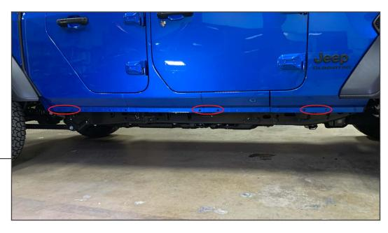
Identify the mounting location of the Rocker Steps on the vehicle. They mount to the pinch welds in (3) locations.
