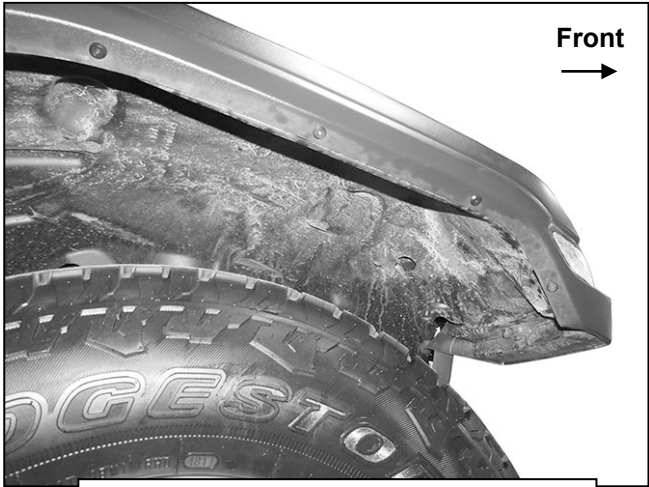
(Fig 2) Remove hardware attaching fender liner to front, top and back of fender (Passenger/Right side pictured)
