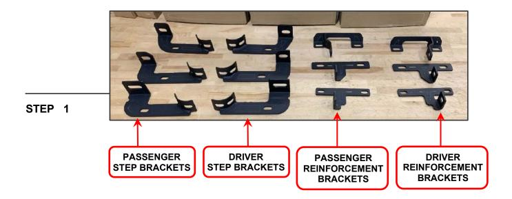
Identify each mounting bracket using the engraved location identifier.
