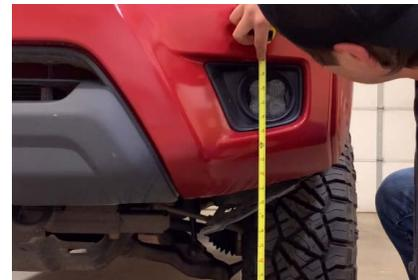
10. On your vehicle, measure the distance between the ground and the center of your SS3 pod. This is your mounting height.
