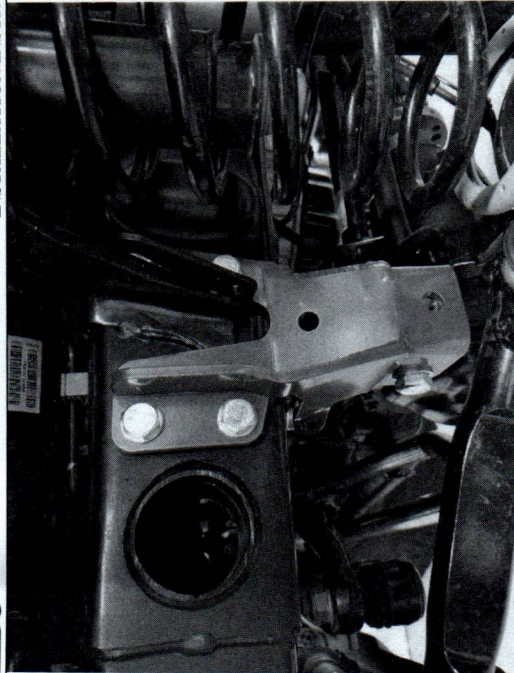
Figure 9. Threading Bolts into Steering Box
