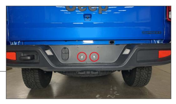
Remove the license plate from the vehicle by removing (2) 10mm screws, then remove (2) 16mm bolts from the bumper. Lift and remove the bumper assembly from the vehicle. Place on a soft workable surface for disassembly.
