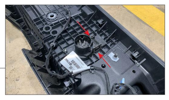
Using a pry tool, press each side of the trailer wiring connector, and remove the connector through the front of the bumper.
