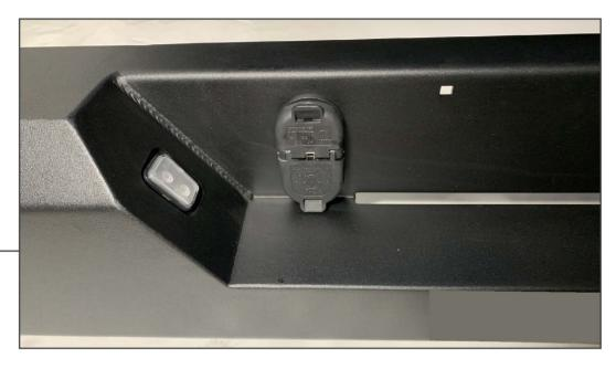
Press the trailer wiring connector into the bumper until fully seated.
