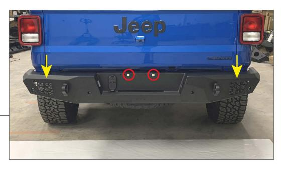
Press the (2) license plate screw retainers into the rear bumper. Secure the vehicle license plate to the bumper using the (2) original 10mm screws.
