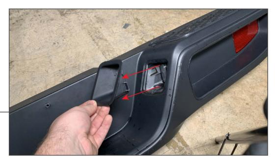
Use a plastic pry tool to remove the outer license plate covers. Then, remove the license plate lamp through the back of the bumper.
