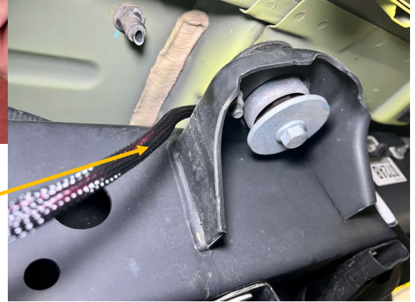
Passenger Side Harness Zip Tie & Cable Clip Anchor Points
