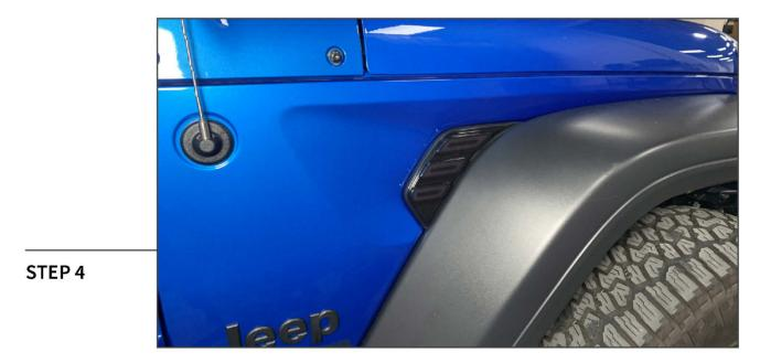
Fit and press the fender light into the vehicle fender.
