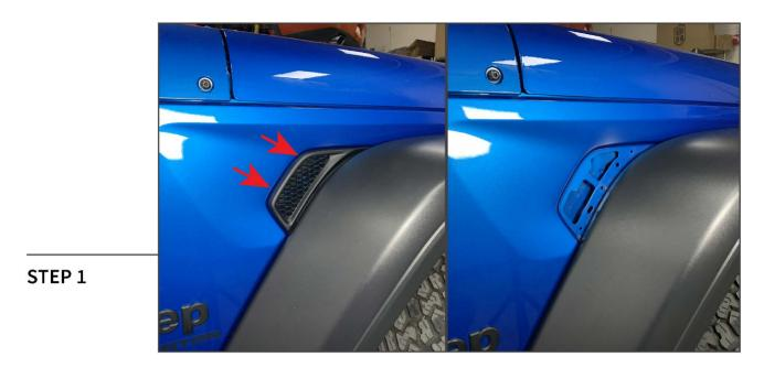
Using a plastic pry tool, pry the vehicle trim panel away from the vehicle.
