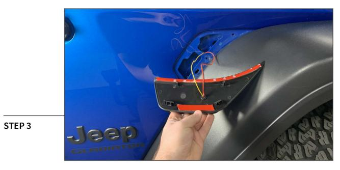
Feed the attached wiring harness through the vehicle fender towards the front of the vehicle. The wiring can be accessed through the engine bay or around the fender liner.
