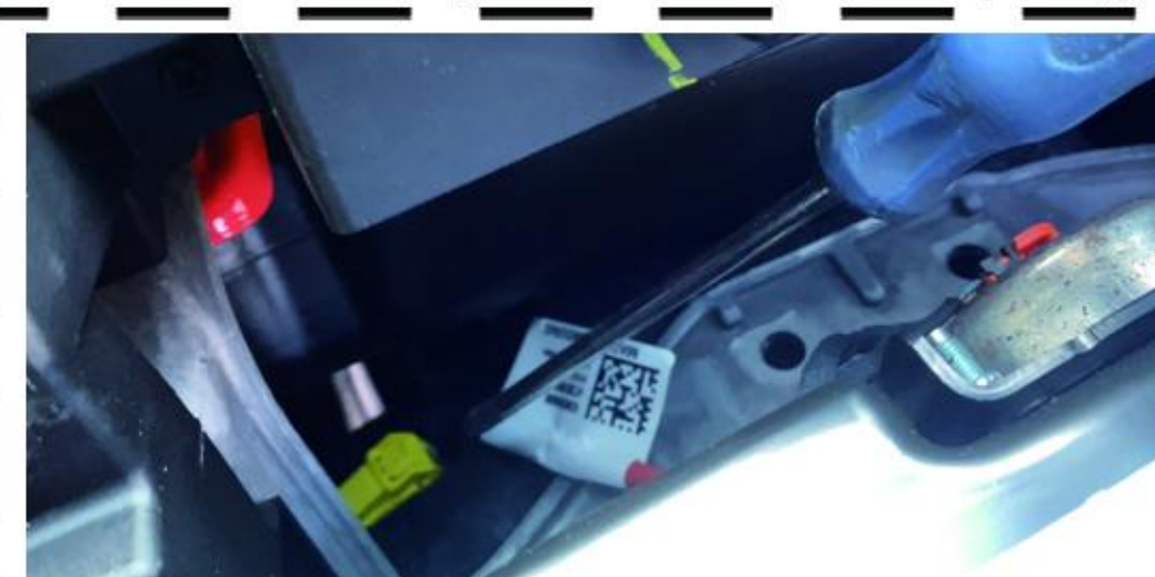
15 When installing the right side panel, Connect the airbag plug (yellow one)
