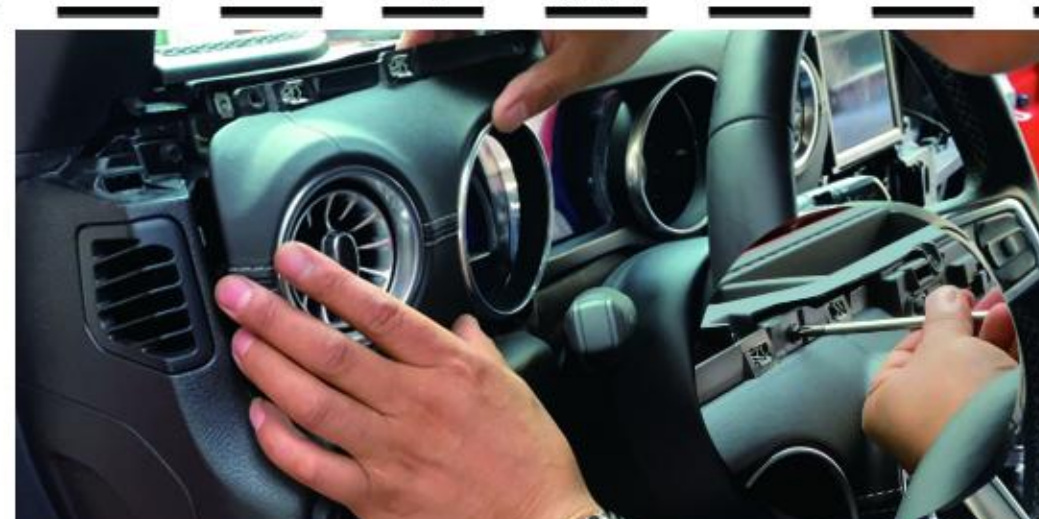
14 Install the panel on. Tighten and fix with screws.
