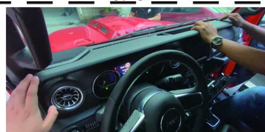
19 Press the strip panel and fix it with screws. Then install the panel from top to bottom.
