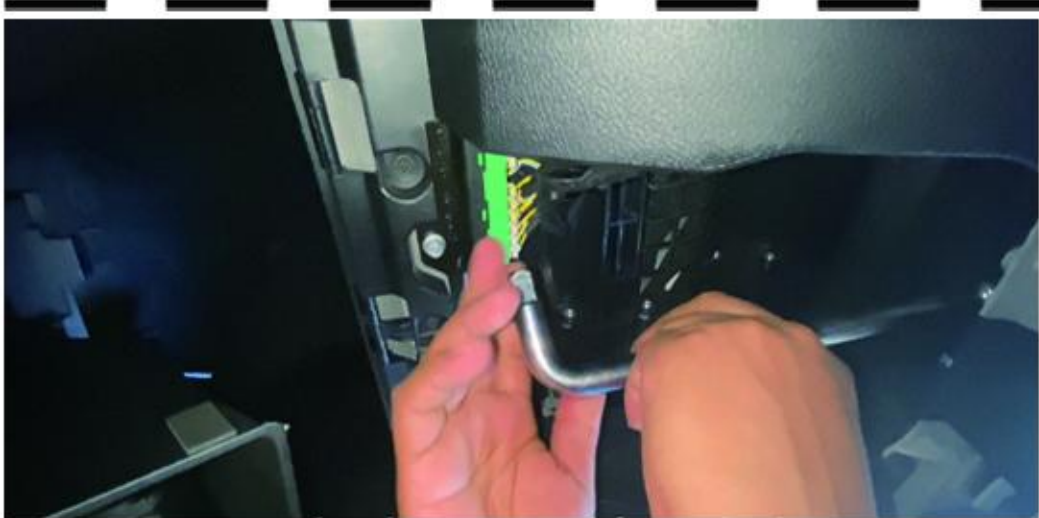
5 2 screws need to be removed from the lower cover plate of the storage box.
