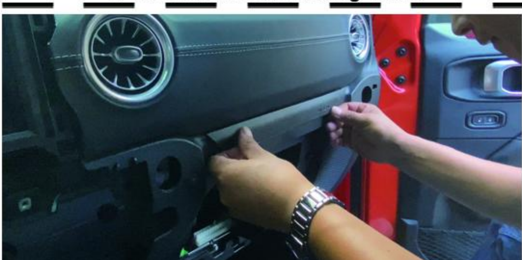
17 Reinstall all panels one by one. As shown, press to install the panel.
