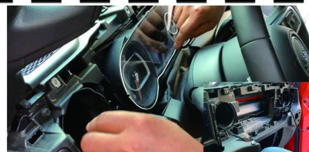
11 And then pull out the line from the other side. Be careful not to get the lines stuck when pulling.
