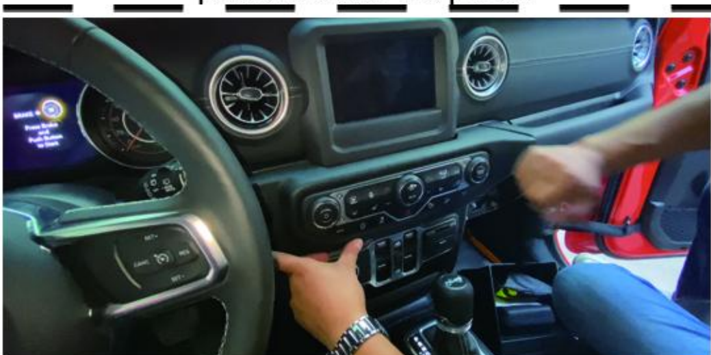
21 Then install the panel from top to bottom.
