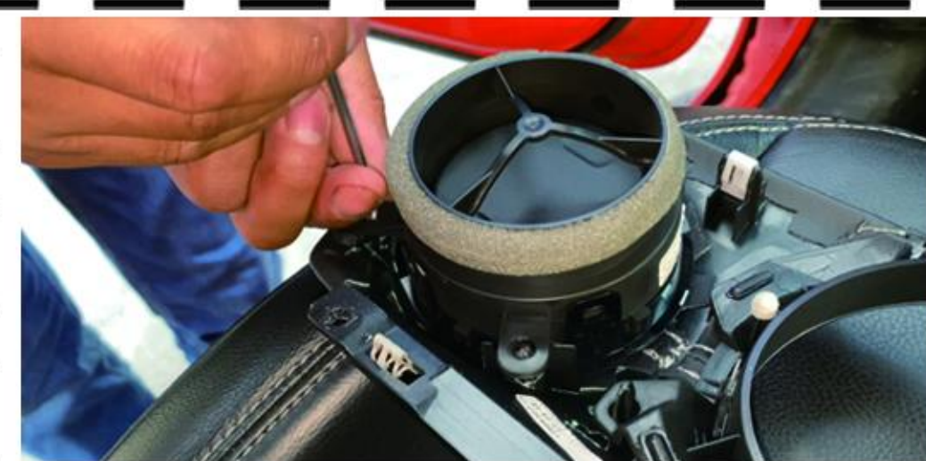
7 Remove the original air conditioning vent.
