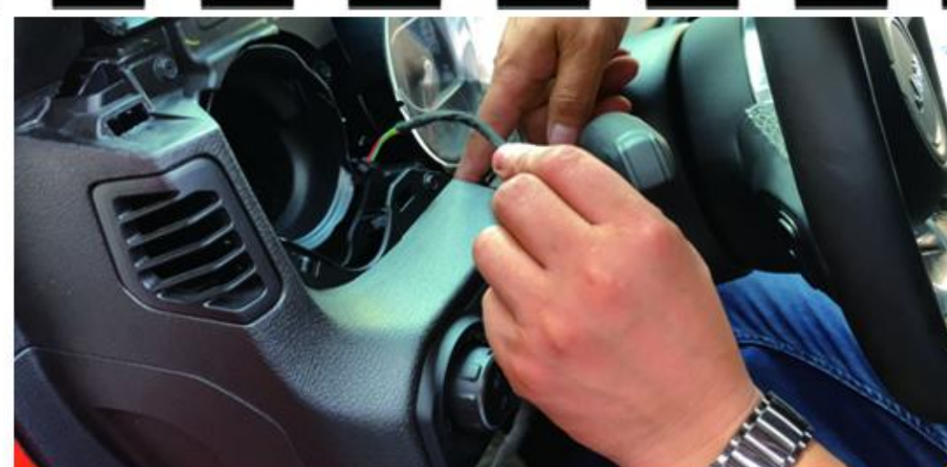
10 As shown, insert the control gas line from the corresponding position.
