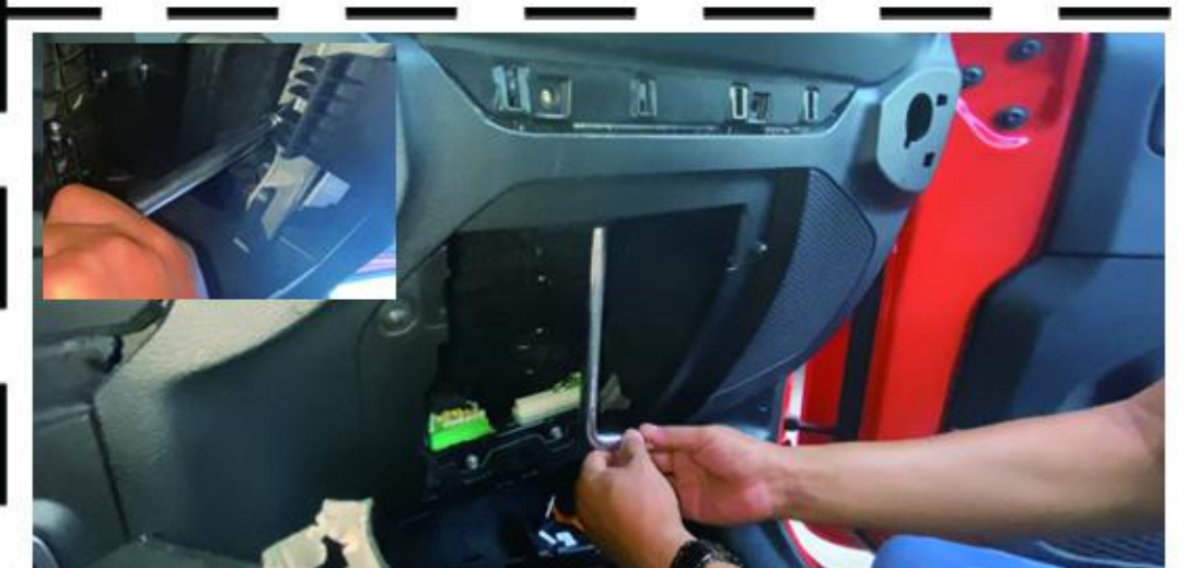
16 Install the two screws inside the storage box.
