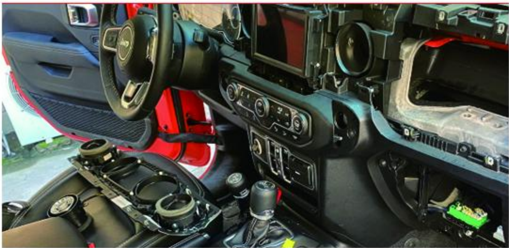
1 Disassemble all cover plates in sequence. Be careful not to damage the panel during removal. (Figure 2 3 4 5)
