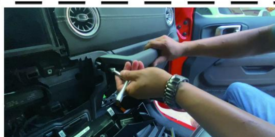
18 Install the armrest and fix it with screws.
