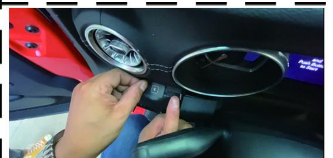
24 Select the desired position and stick the switch on the panel.
