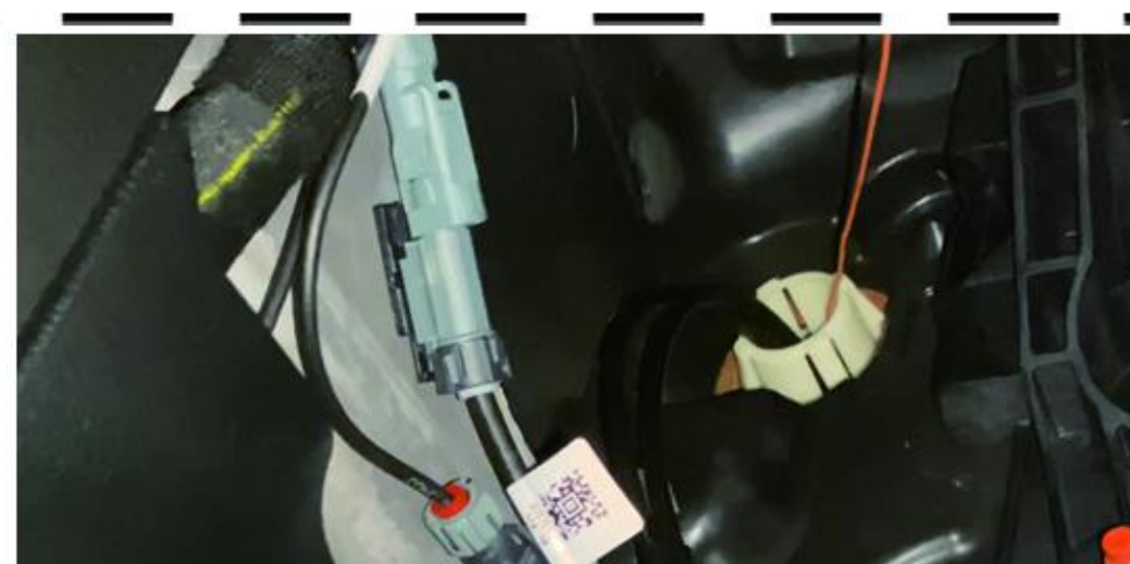
26 Run the red line through the hole to the ACC Fuse box.
