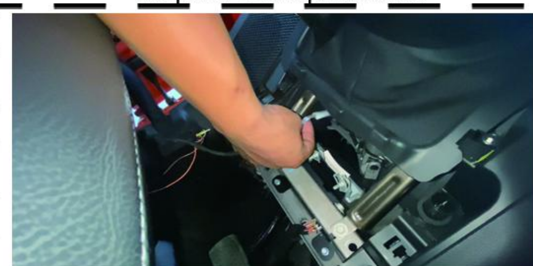
23 Thread the controller wire in from the bottom.
