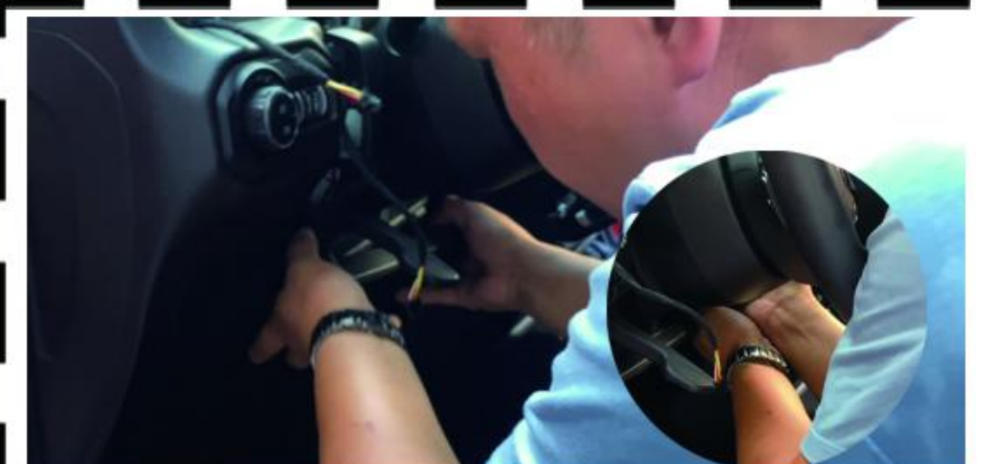
12 Insert the line of the control box from the bottom.
