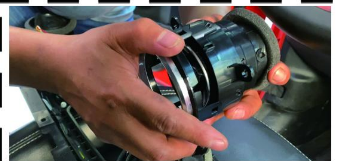
8 Remove the silver fixing ring on the original air conditioner vent and install it on the new air conditioner vent.
