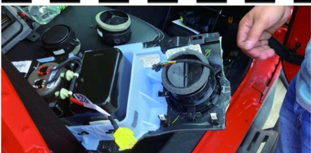
9 Install to the corresponding LHC/LHO/RHC/RHO. Tighten the screws in turn. (Pay attention to the correct installation direction)
