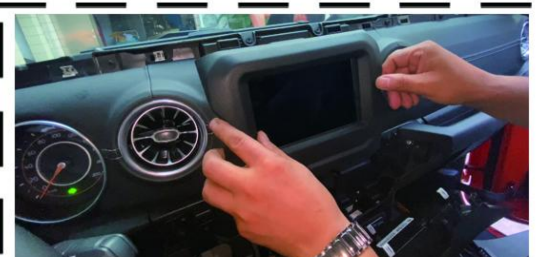
20 As shown, press to install the panel. Fix it with screws.
