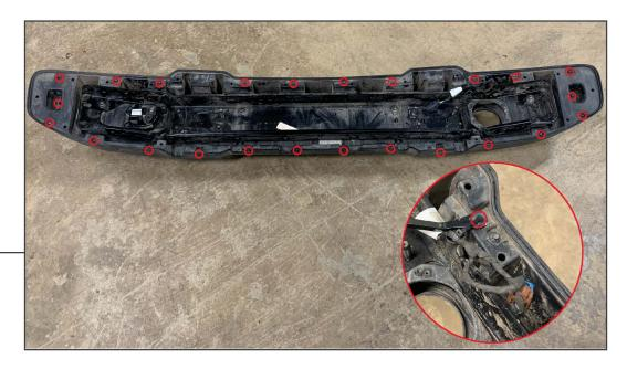
Remove the factory wiring harness from the bumper by separating the bumper into (2) pieces by removing the screws around the outer edge of the bumper. Unclip the wiring harness and transfer it to the new bumper.
