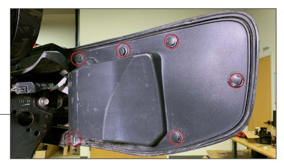
Begin by removing the outer bumper covers. Using a soft pry tool, remove the (6) plastic push clips.
