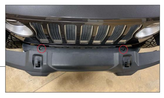
Remove the (2) plastic clips securing the bumper filler panel to the vehicle.
