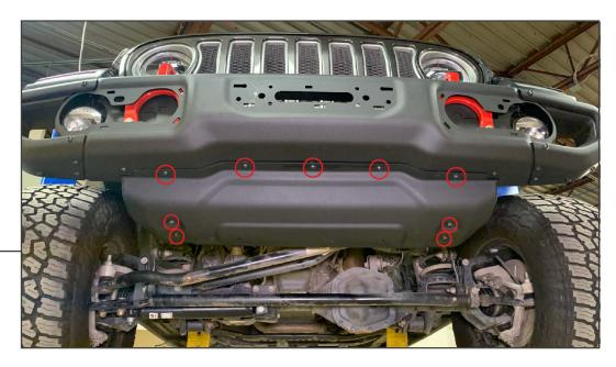
Install the skid plate to the vehicle. From behind, bolt the skid plate brackets to the inner frame rails using (2) M10x1.50 30mm bolts, (2) M10 washers per bracket. These will bolt into the hexagonal rivnuts from Step 11. Screw the front edge of the skid plate into the bumper using (5)M8x1.25 35mm bolts, and flat washers.
