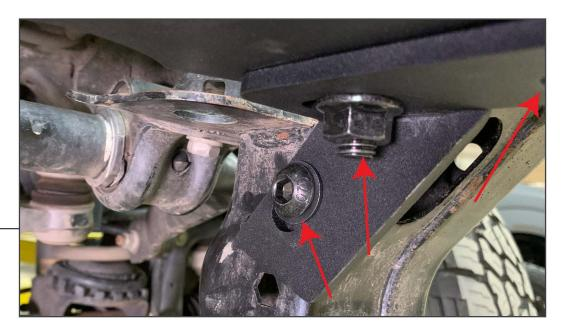
Mount the winch plate to the winch plate brackets using M12 (2) M12x1.75 30mm bolt, (2) washers, (2) flange nuts per bracket. Mount the winch plate to the vehicle using (1) M12x1.75 30mm bolt, (1) flat washer, (1) flange nut per bracket.
