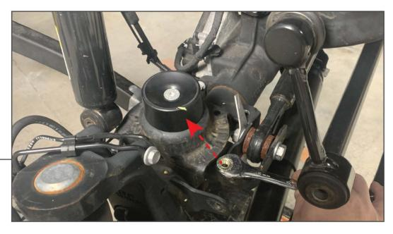
Locate the pre-drilled hole in the axle spring perch. Secure the (1) bump stop to the vehicle axle using (1) M10 x 60mm Tapered Allen bolt and (1) M10 flange nut. Tighten until secure.
