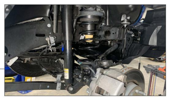
Lift the vehicle axle using a floor jack. Take note to the dowel pin alignment, as well as other components while lifting. Re-install all the original vehicle components to the vehicle following steps 1-4 in reverse order. See last page for torque specifications. Leave the track bar unbolted until the end of the installation.
