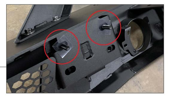
Fit the (4) M12 stud plates into the bumper mounting pad, and hold into place using the (4) M12 plastic stud holders. This will allow the studs to remain in place while mounting the bumper.
