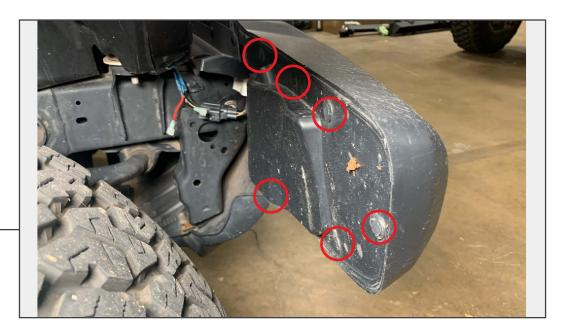
Remove (6) plastic push clips from the bumper end cap cover. Repeat this procedure to the opposite side of the vehicle.
