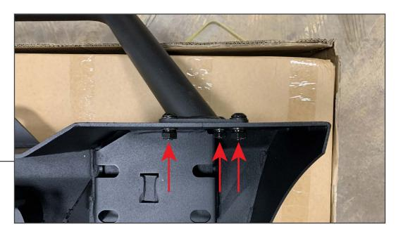
Place the new bumper on a workable surface. Install the (1) Over-Rider Bar to the bumper using (6) M10x1.50 x 35mm Hex bolts, (6) M10 lock washers, (12) M10 flat washers, and (6) M10 nuts. Tighten until secure.
