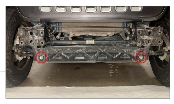
**Optional:** Remove (2) 16mm bolts from the lower metal shield, then lift upwards to unhook the shield from the vehicle.
