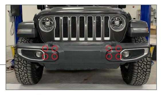
From behind the bumper, remove (8) 18mm nuts to release the bumper. Once all hardware is removed, pull the bumper away from the vehicle.
