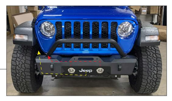
Neatly route the fog light wiring harness away from any moving/hot components, then plug the harness into the vehicle wiring harness connector.
