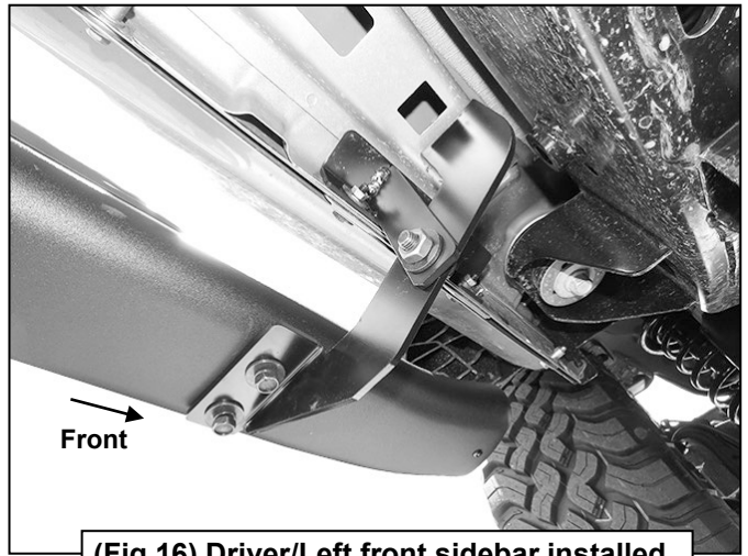
(Fig 16) Driver/Left front sidebar installed
