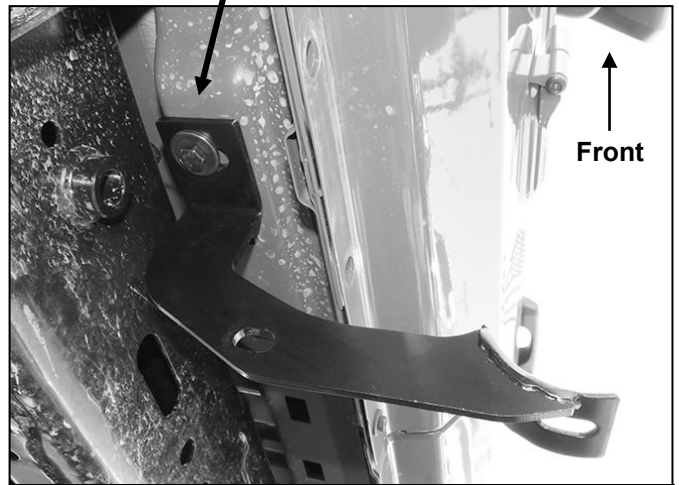
(Fig 4) Driver/Left front Mounting Bracket installed
