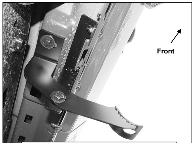
(Fig 6) Driver/Left front Brackets installed
