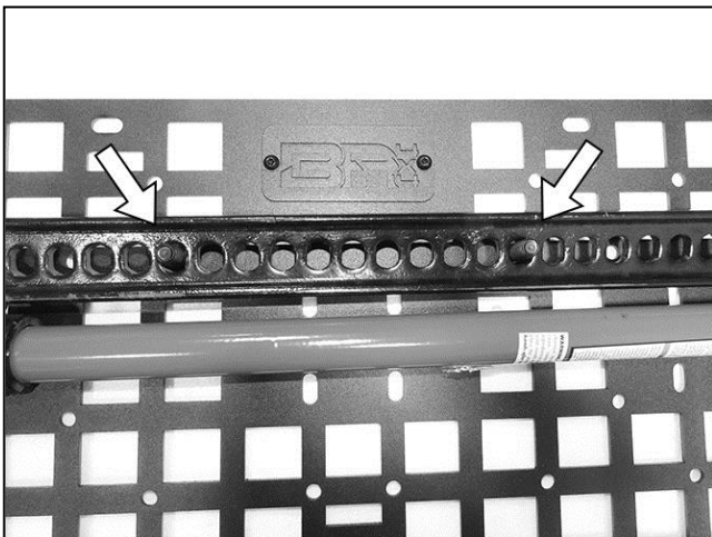
(Fig 7) Example of beam style recovery jack attachment to Carriage Bolts in Panel (arrows)
