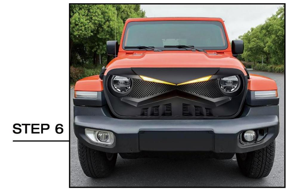
Fix all the bolts and finish the installation of new grille.
