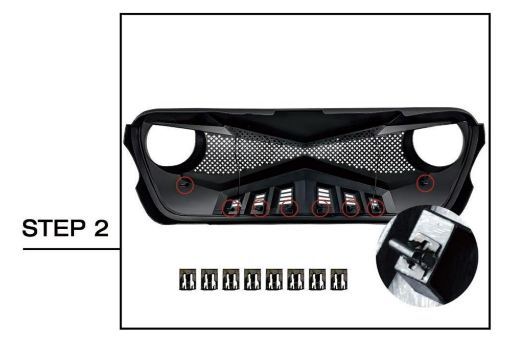
Install the retaining clips(8) in the appropriate position on the back of the grille.
