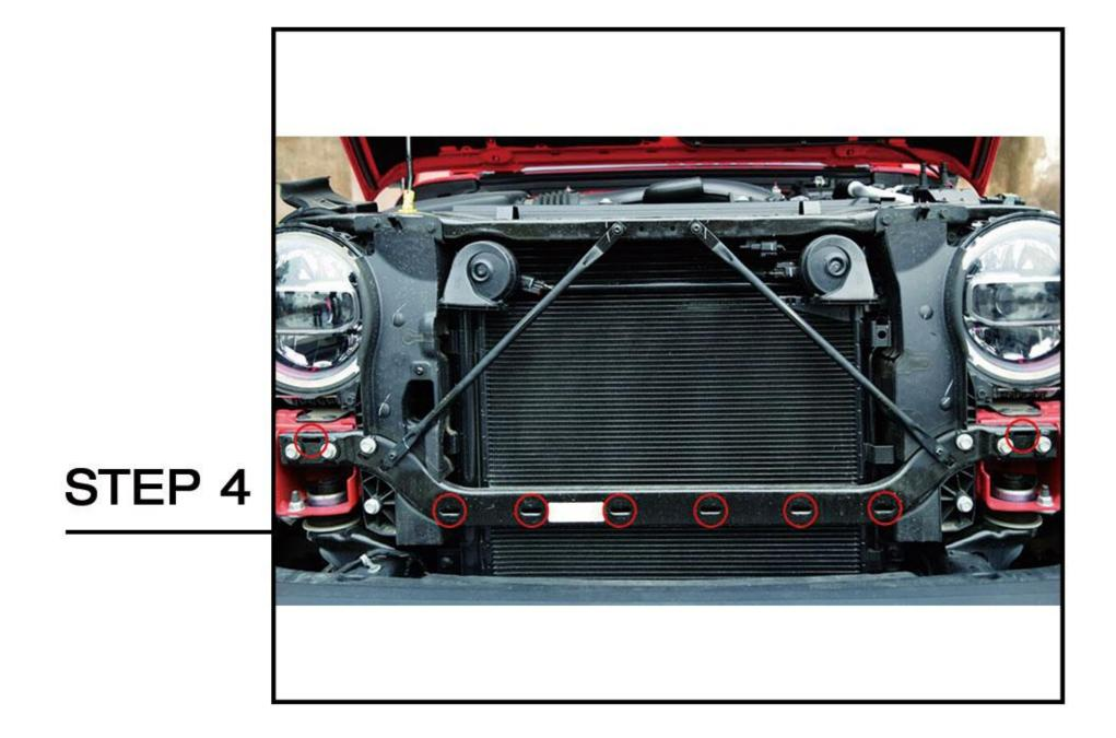
Align the supplied retaining clips(8) on the grill with the corresponding holes on the car and push inwards. Fix the grille to the car.
