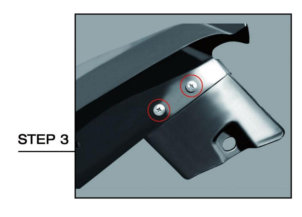
Fix the bracket with screws.
