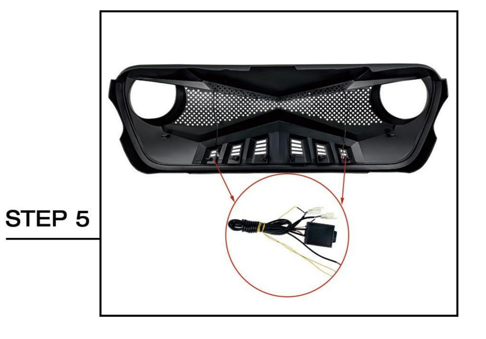
Wiring: Connect the two connectors to the harness drive control box. The red wire connects to the ACC, the black wire connects to the negative of battery, and the yellow wire connects to the turn signal.
