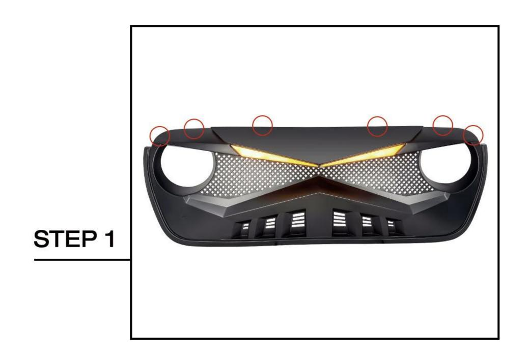
Using a panel removal tool, remove the(6) push clipsholdingthe grille cover to the vehicle. Pull the grille cover from the vehicle.
