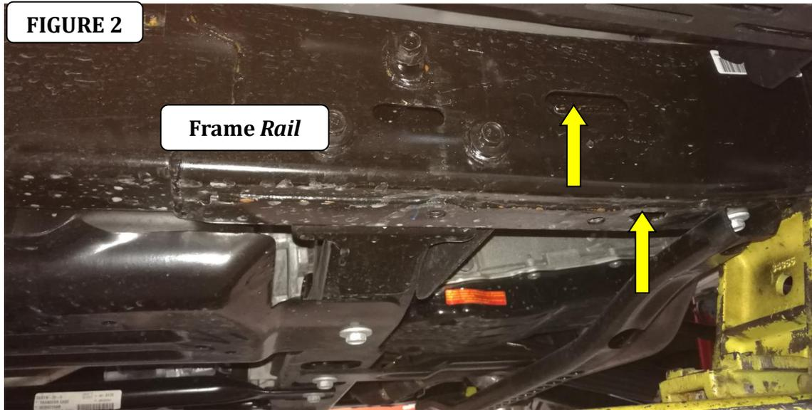
**Step-2** At the front location, thread a bolt plate in the guide bolt then introduce it through the obround hole, the tip of the bolt guide must come out through the bottom hole of the frame rail. Do not pull out the bolt plate attached to the bolt guide. Place another bolt plate in the obround hole and use a vinyl gasket to prevent the bolt plate from falling into the frame rail, (FIGURE 3 & 4).
