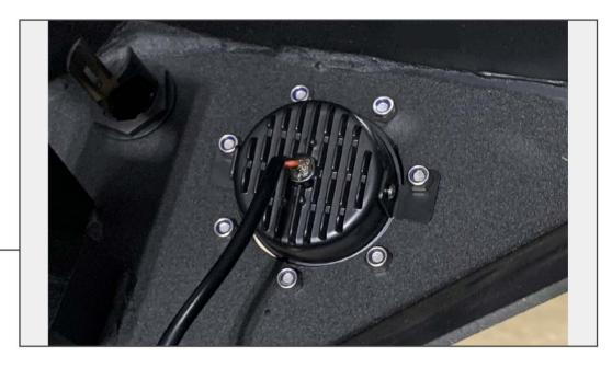
Using (34) M6 Allen bolts and (34) M6 lock nuts, secure the (4) LED lighting to the vehicle bumper. With all of the lights mounted, plug in the wiring harnesses.
