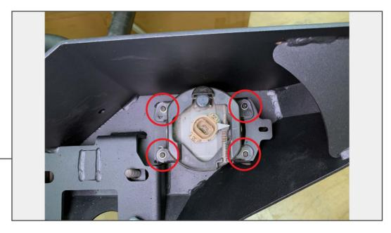
Using (4) M4 Allen bolts, (4) M4 lock washers, (4) M4 flat washers, (4) M4 nuts, attach the fog light to the previously installed fog light bracket. Repeat for the opposite side fog light.
