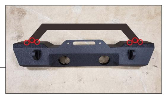
Place the bumper on a soft surface for component assembly. Install the over rider bar to the top of the bumper using (6) M10 bolts, (6) M10 lock washers, (12) M10 flat washers, and (6) M10 nuts. Tighten until secure.
