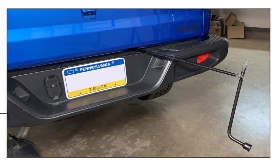
With the vehicle on the ground, lower and remove the vehicle spare tire using the tools included with the vehicle (under the rear seat). This allows for maximum clearance to remove the original exhaust.
