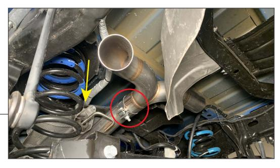
Install the (1) "T" pipe to the previously installed front exhaust pipe, loosely secure with the previously placed (1) 3" exhaust clamp. With the "T" pipe in place, secure the rear exhaust hanger to the vehicle frame.
