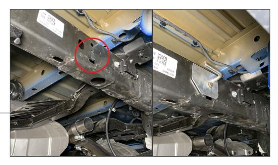
Install (1) M8 clip nut into the RH side vehicle frame. Mount the hanger bracket to the frame using (1) M8 bolt. Ensure the hanger is pointing towards the rear of the vehicle, and tighten the bolt to secure into place.
