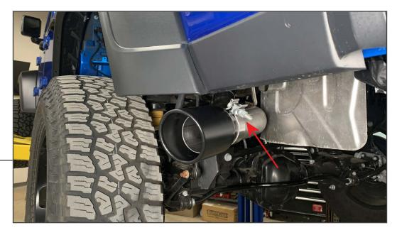
Install the exhaust tip to the rear exhaust pipe, and loosely secure using the previously placed (1) 3" exhaust clamp.
