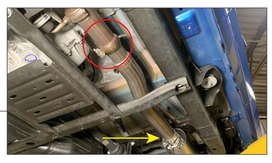
Align the (1) front pipe to the vehicle, and loosely secure using the original ball flange clamp.
