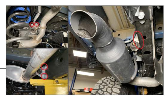
Locate the (3) exhaust hangers along the exhaust system. Remove the (2) 13mm bolts from each hanger to disconnect the exhaust system from the vehicle.
