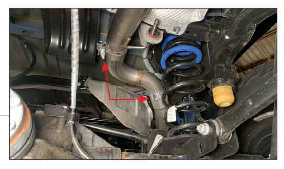
Install the (1) "S" pipe to the previously installed exhaust pipe, loosely secure with the previously placed (1) 3" exhaust clamp.
