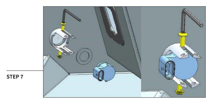
**Optional Sensor Mounting:** Using the provided M4 Allen screws lightly tighten the screws into the sensor to hold it in place.
