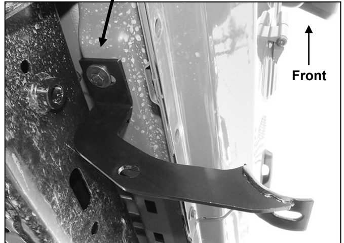
(Fig 4) Driver/Left front Mounting Bracket installed
