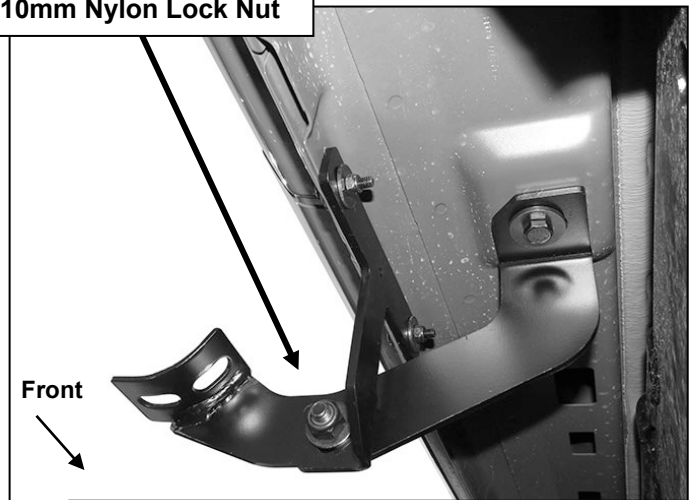
(Fig 10) Driver/Left Center Brackets installed
