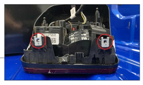
Remove the (2) screw clips using a flat head screwdriver, and transfer the clips to the new tail light.
