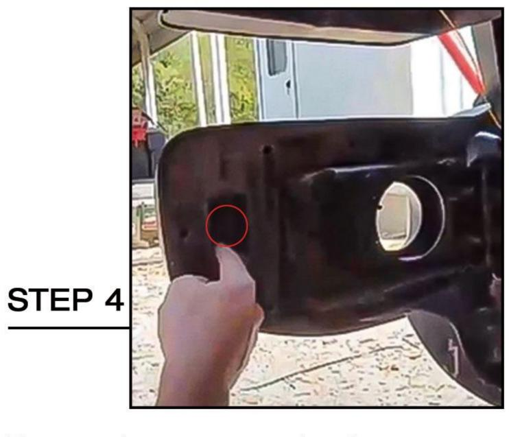
Remove the screw securing the bumper cover.
