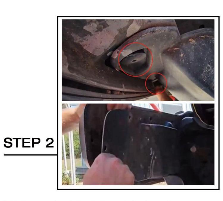
Remove the bottom two bolts, then remove the plastic cover.
