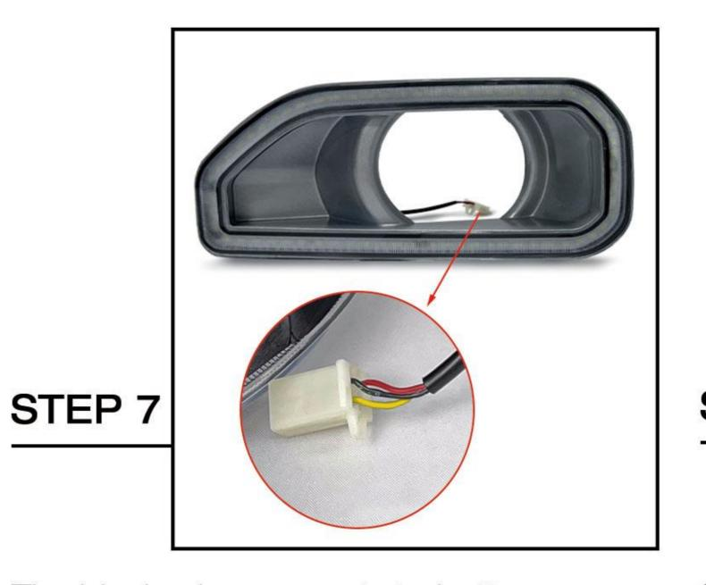
The black wire connects to battery negative. The yellow wire connects to turn signal lights. The red wire connects to ACC.
