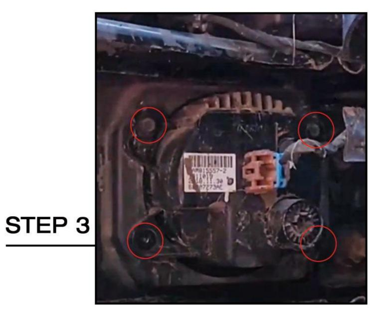
Remove the four screws fixed on the back of the fog lights, unplug the wire harness, and take off the fog lamp.
