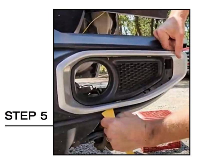
Remove the original bumper fog light cover. Install the new LED bumper cover.
