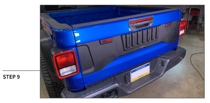
Re-install the vehicle tail light and the tailgate panels using the original hardware.
