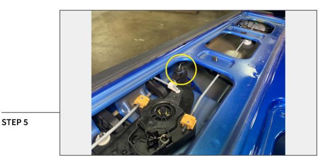
Unplug the 3rd brake light connector from the third brake light. Splice the (2) wires into the parking light following the diagram below. Once spliced, plug the connector back into the 3rd brake light. Note: Temporarily disconnect wiring retainers to allow wiring flexibility.
