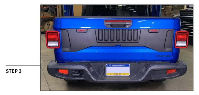
Route the tailgate trim panel wiring through the 'P' alignment hole. Familiarize the alignment of the panel onto the vehicle prior to tape removal. Once familiar, peel the red tape backing from the tailgate panel and adhere the panel to the vehicle. Apply firm pressure to ensure proper adhesion.
