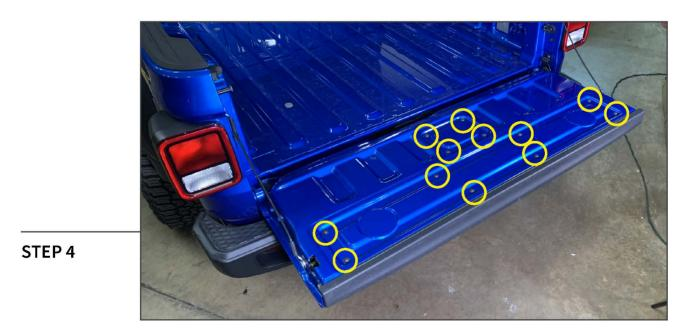
Remove (12) T-30 Torx screws from the inner tailgate panels and set the panels aside.
