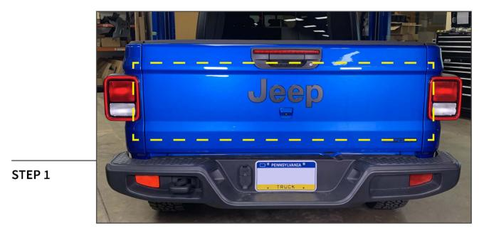
Clean the vehicle tailgate using isopropyl alcohol and a microfiber cloth.
