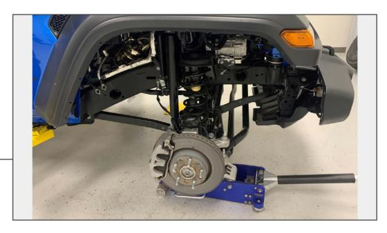
Lift and support the front of the vehicle using a jack and jack stands. Remove the front wheels from the vehicle. Place the floor jack under the lower control arm mount on the axle to relieve suspension tension.
