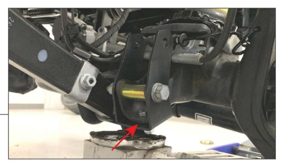
Install the shock absorber bracket to the lower shock mount using the original 18mm bolt and (1) bolt sleeve. Install (1)  $5/16-18 \times 1$ " bolt, (1) 5/16 flat washer, and (1) 5/16-18 lock nut through the bottom of the bracket.
