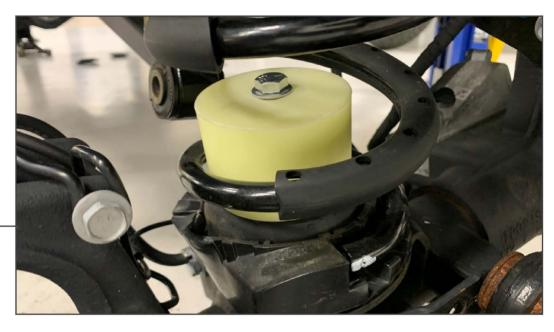
With the bump stop extension inside the coil spring, install the coil spring into the vehicle. Secure the bump stop extension to the axle using (1)  $5/16-24 \times 3$ " bolt, (1) 5/16 flat washer, and (1) 5/16 lock nut.
