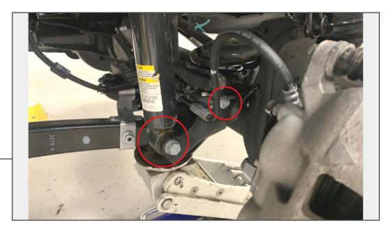
Remove the 18mm lower shock mounting bolt from the axle. Remove (1) 10mm bolt from the brake line bracket under the spring perch.
