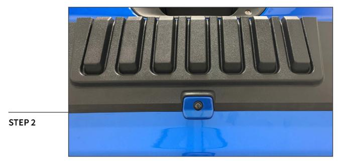
Familiarize the tailgate trim panel on vehicle by aligning the lower cutout with the back-up camera on the vehicle.
