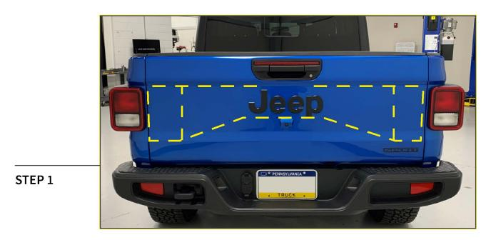
Clean the vehicle tailgate using (2) alcohol prep pads.
