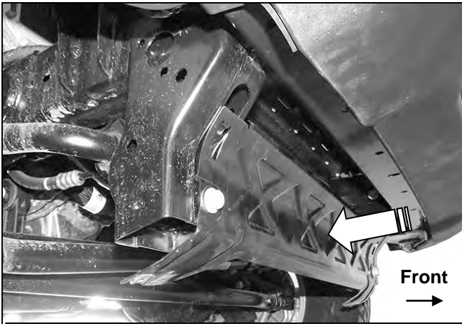
(Fig 1) Remove splash guard and bracket (arrow)
