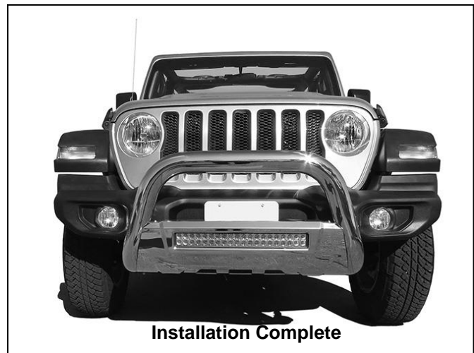
(Fig 10) Attach Tyger Guard with Brackets to the outside of the Frame Mounting Brackets
