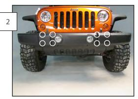
Remove the 4 nuts on the backside of the bumper that attach the front bumper to the frame.
