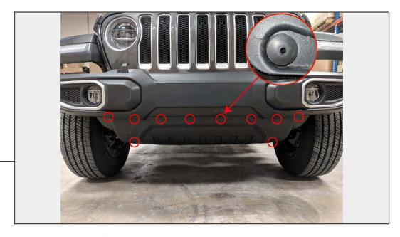
From under the vehicle, remove the (8) plastic push pins securing the factory splash shield to the vehicle. Next, remove the (2) 8mm screws and remove the splash shield from the vehicle.
