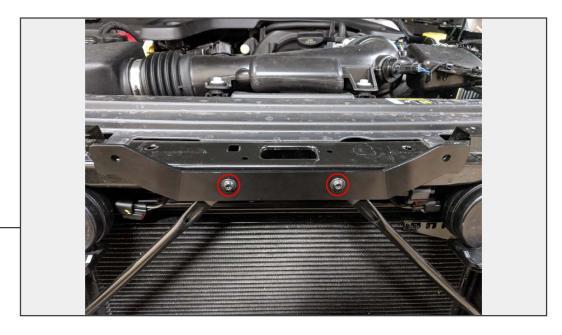
Re-install the factory radiator support braces, and the middle grille bracket using the factory T-30 Torx screws.
