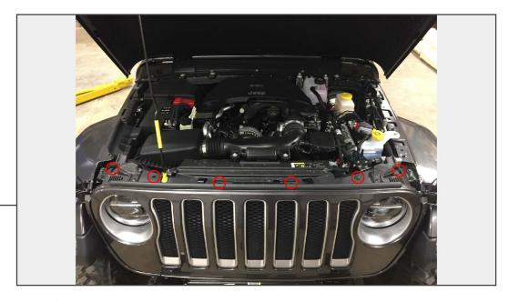
Locate, and remove the (6) push pins holding the grille in place. Gently pry the lower part of the grille away from the vehicle, and remove the grille completely.
