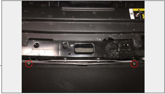
Align the grille with the holes in the middle grille bracket. Secure the grille to the middle grille
