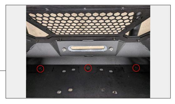
With the upper part of the grille installed, secure the lower part of the grille to the bumper using the (3) M8x30mm bolts, (6) flat washers, and (3) lock nuts.
