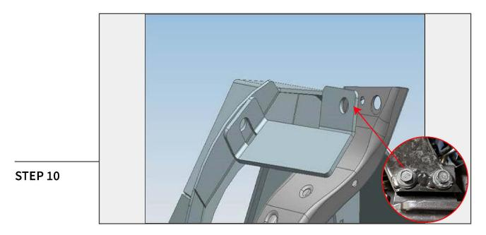
Locate the factory 13mm radiator support bolt, and remove from the vehicle. Install the corner bracket to the radiator support using the factory bolt. Then, install the corner part of the grille to the bracket using the (1) M6 screw, (2) flat washers, and (1) lock nut.
