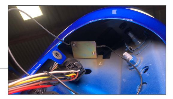
Plug in the tail light, push the light into the vehicle. Secure the light to the vehicle using the factory hardware.
