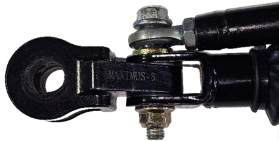
Permanent Bolt Setup (1/2" Hex Bolt)
