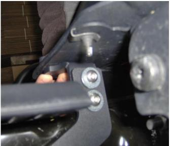
**4- Install the Striker Bar & LED Light Brackets:**Place the Striker bar on the mounting locations on the bumper and align the front hole to corresponding mounting points on the bumper and insert the back stud (welded bolt) through corresponding holes on the bumper and reinforcement brackets you installed in step 3 (make sure the reinforcement brackets are loose enough to allow adjustment).
