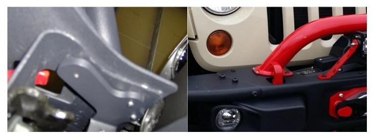
Align and tighten front bolts and back nuts. Make sure the bar is seated flat on the mounting surface. Now tighten the lower M8 hex bolts of the reinforcement brackets, 1 on each side.
