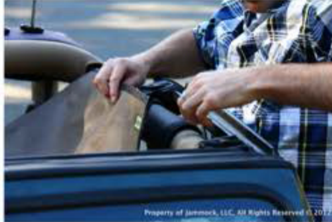
2.) 1987-2006: Slide webbing around the driver's side roll bar
