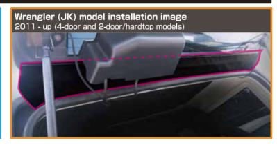
(1) Pull the weather strip at the top of the rear window towards you to remove it until the left and right corner joints are visible.
