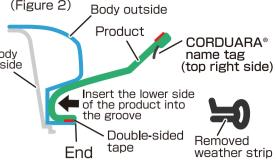
(3) Align the Wrangler (JL) and (JK) with the joint positions on the left and right, respectively, before installing this product. Attach the product to align along the edge on the upper side where the weather strip has been removed while peeling off the (white) release paper. (Figure 2)
