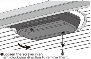
Remove the rear wiper motor cover on the vehicle.
