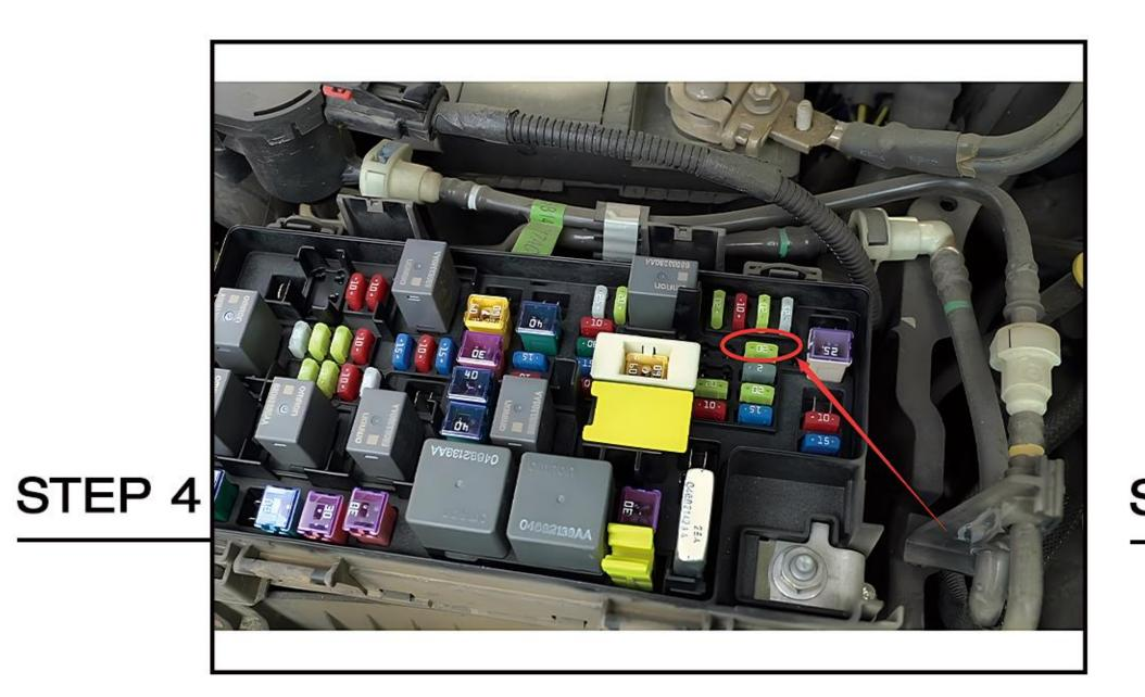
Connect the red and black wire of the light bar to ACC and negative of battery.
