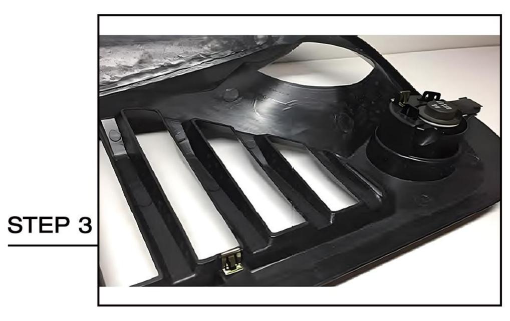
Press on the (6)supplied retaining clips. Using the factory grille as a reference, apply the supplied weather stripping acrossthe top of the grille.
