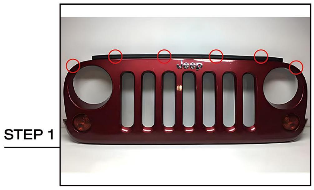
Using a panel removal tool, remove the (6) push
