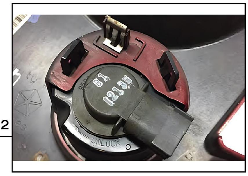
Remove the factory turn signals by unclipping them from the factory grille. Transfer them to the new grille.
