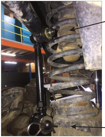
Bolt up link to swaybar with nyloc nut and M12 washer - place washer between swaybar ball joint (not under nut)
