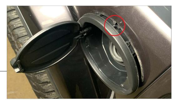
Align the locating tab on the new fuel door with the vehicle alignment slot. Carefully press the new fuel door over the fuel filler neck and on to the vehicle. Firmly press the fuel door to the vehicle to engage all mounting clips.
