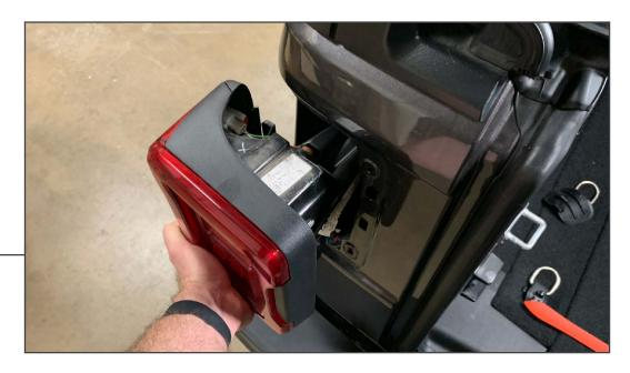
Pull the tail light away from the vehicle to access the light's wiring connection.
