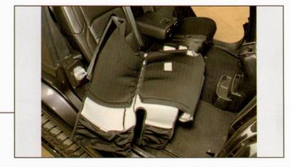
Identify the large rear upper seat back. Unzip, and separate the top and bottom portions of the seat cover.
