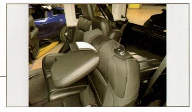
Slide the seat cover over the seat back. Tuck the center section of the cover through the headrest posts. Connect the hook and loop on the top of the seat cover.
