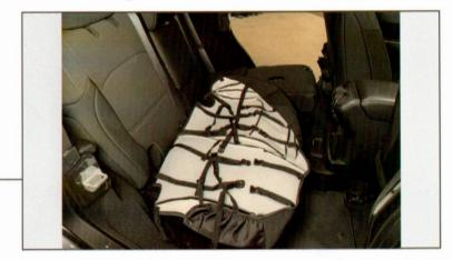
Identify the larger portion of the seat bottom. Disconnect the straps. Feed the straps through to the backside of the seat.
