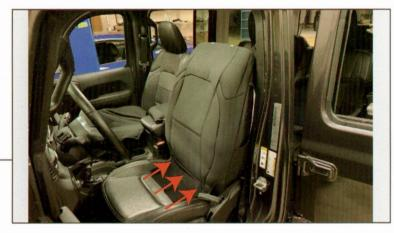
Wrap the soft portion of the upper seat cover through the seat back. \*\*Note: Folding the seat forward allows for more space between the seat back and seat bottom.
