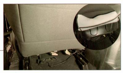
Fold the seat back bottom from Step 4 under the seat cover. Then pull the soft portion of the seat cover from Step 5 up the back of the seat and attach the front and rear portions of the seat cover together.
