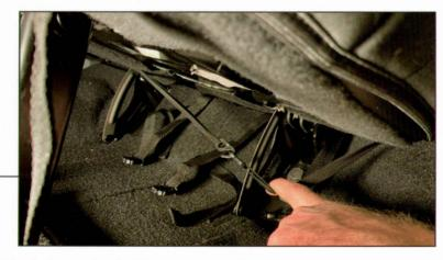
Latch the elastic hooks from each side of the seat cover together.
