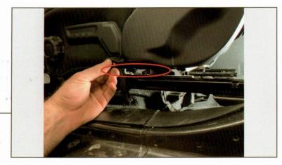
Route the side straps under the seat by feeding them through the gap between the seat bracket and the slider. Location will vary from side to side. Ensure the strap is above the seat slider otherwise the slider may damage the strap.
