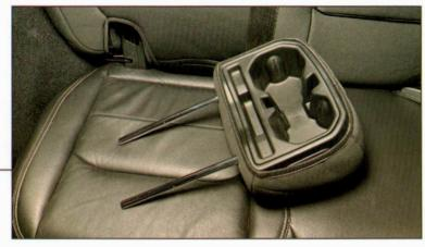
Locate the smallest remaining headrest cover. Insert the headrest posts through the cover, then wrap the cover around the headrest.
