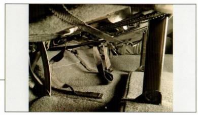
Reconnect the straps from the front of the seat cover to the straps on the rear of the seat cover. Tighten the straps for desired fit.
