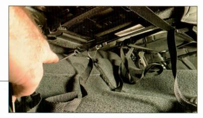
Latch elastic hooks from each side of the seat cover to one of the center straps.
