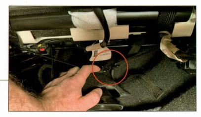
From under the seat, hook both side straps together.
