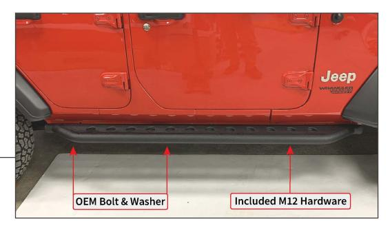
With assistance, lift the rock slider assembly to the vehicle frame.
