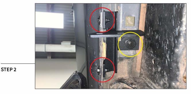
Place the front pinch weld bracket to the vehicle. Loosely install (1) M8 bolt, (1) M8 lock washer, and (1) M8 flat washer through the pinch weld bracket into the pre-drilled/threaded hole in the vehicle.
