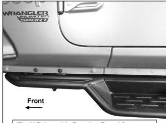
(Fig 9) Driver side Running Board-front attached to the <u>back</u> side of the pinch weld
