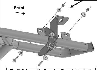
(Fig 8) Driver side Running Board attached to the <u>back</u> side of the pinch weld illustrated
