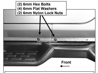
(Fig 10) Driver/left side Running Board-center attached to the <u>back</u> side of the pinch weld
