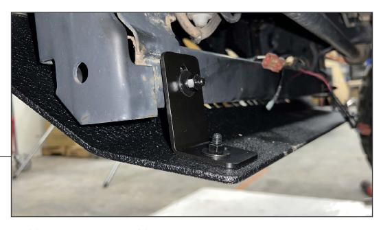
Fit (1) M8 flat washer, (1) M8 lock washer, and (1) M8 nut onto the M8 stud plate loosely. Then, loosely secure the mounting bracket to the skid plate using (1) M8 x 30mm Allen bolt, (1) M8 lock washer, (2) M8 flat washers, and (1) M8 nut.
