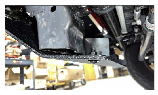
Loosely secure the skid plate to the previously mounted bracket using (1) M8 x 30mm bolt, (1) M8 lock washer, (2) M8 flat washers, and (1) M8 nut. Add (1) spacer in between the bracket/skid plate per side, if desired.
