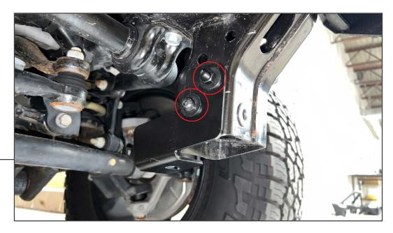
Using the photo reference above, fit the LH/RH mounting brackets to the vehicle frame using (2) M8 flat washers, (2) M8 lock nuts, (1) M8 x 30mm bolt, and (1) M8 nut.
