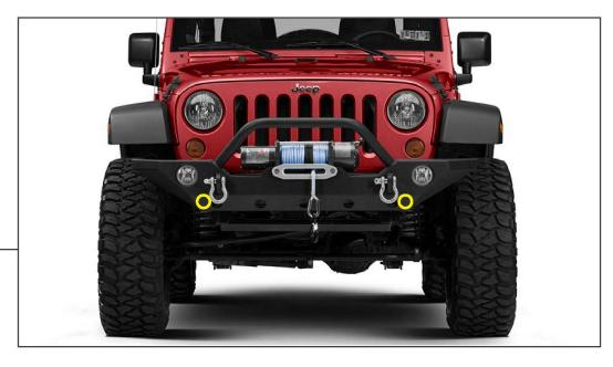
Remove the lower outer corner 18mm bolt & washers from each side of the bumper.
