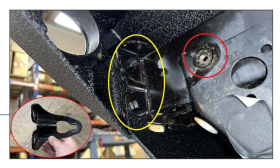
Identify if the OEM outer bumper brackets are in place. If the outer brackets are still attached, remove the (2) 18mm bolts/nuts, and remove (1) 16mm bolt from the vehicle frame. Remove the bracket and set aside.
