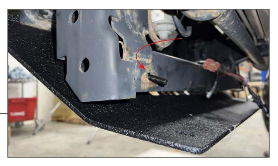
**Wrangler JK:** Using (1) M8 stud plate, guide the stud through the lower frame through the hole. Repeat this step for the opposite side of the vehicle.
