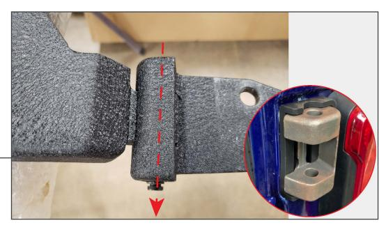
Using a large hammer, carefully hammer in the hinge pin to install the door hinge to the carrier. Then, secure the pin using the metal 'C' clip. Place the provided hinge gasket over the hinge prior to installing it to the vehicle.
