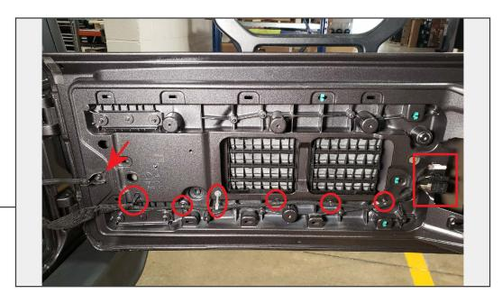
Using a trim panel removal tool, carefully pry the plastic push clips securing the factory wiring to the tailgate. Then, use a T-40 Torx bit to remove the door hinge stop from the tailgate.
