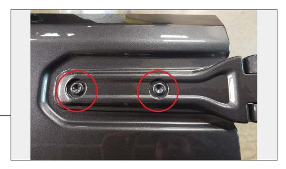
Carefully lay the tailgate down on a soft and flat working surface. Remove the (2) T-50 Torx bolts from each hinge. Remove both brackets from the tailgate.
