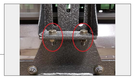
Install the lower part of the third brake light bracket to the carrier using the (2) M10x1.50x30mm bolts, washers, and lock nuts.
