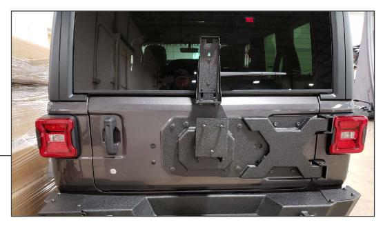
Reinstall the tailgate using the factory hinge hardware from Step 12.
