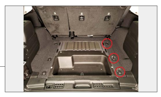
Locate and remove the (3) passenger side anchor hooks using a T-40 Torx bit. Then, remove the anchor hook panel.
