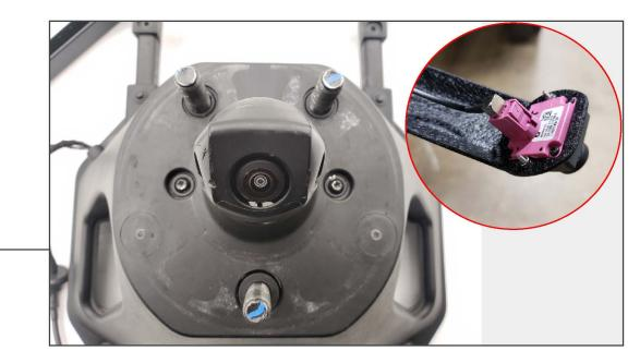
Remove the (2) T-25 Torx screws from the original tire carrier. Pull the camera mounting assembly through the rear of the tire carrier. Unplug the connector, and remove the T-9 Torx screws securing the camera to the bracket. Transfer the camera to the new bracket using the (2) M2 screws, washers, and nuts.
