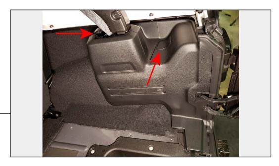
Using a trim panel removal tool, pry and remove the seat belt trim cover and taillight access cover.
