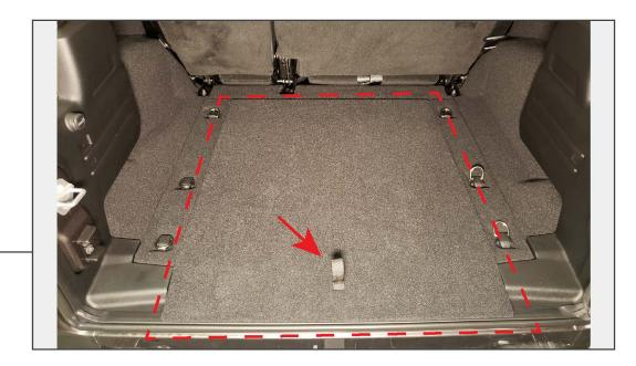
Pull and remove the rear trunk cover from the cargo area.
