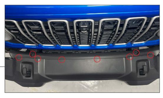
Using a panel removal tool, remove the (8) plastic push clips securing the trim panel between the grille and front bumper. Remove the trim panel from the vehicle.
