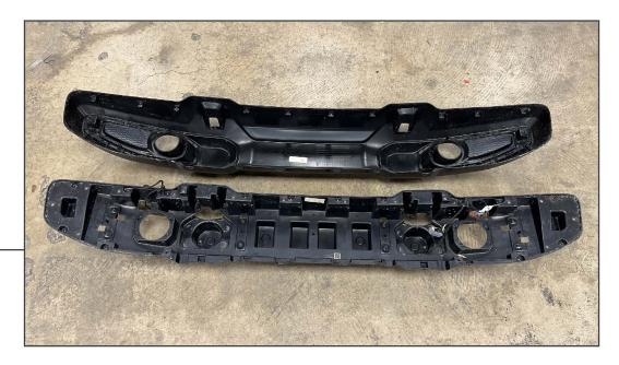
Lift the rear portion of the bumper away from the front portion. Use a panel removal tool to release all of the fog light harness retainers.
