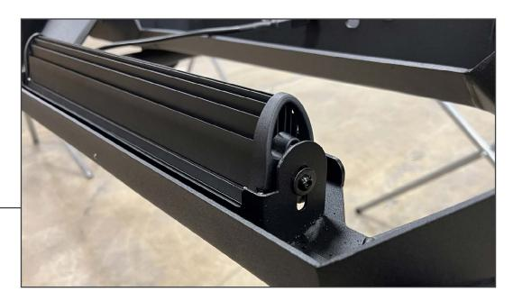
Light Bar Installation: Fit the light bar to the bumper with the wiring harness to fit on the passenger side of the vehicle. Secure the light bar to the bumper over-rider bar using (2) M6 x 16mm bolts, (2) M6 lock washers, and (2) M6 flat washers.
