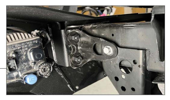
With a helper, lift the bumper to the vehicle frame rails. Loosely fit the bumper to the vehicle, and adjuster/center the bumper into place. If desired, re-install the reinforcement plates using the original hardware (install one side at a time, expand bolt holes if necessary).
