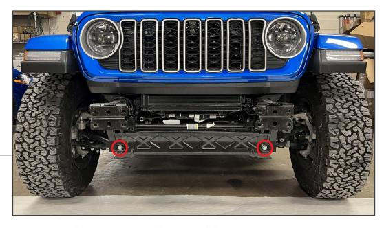
If installing the lower skid plate (SKU # J127064-JL), remove (2) 16mm bolts from the lower splash plate.
