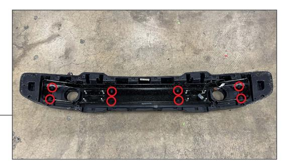
Remove (8) 15mm nuts from the metal bumper core. Then, lift the core away from the bumper.
