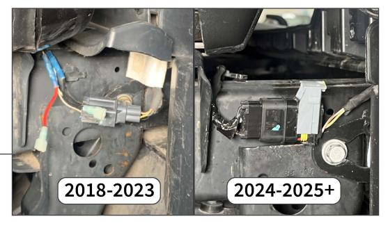
Locate the fog light wiring harness connector along the passenger side frame rail.
