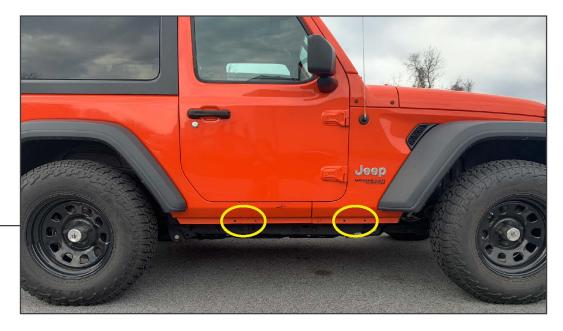
Begin by locating the (2) pinch weld mounting locations under the vehicle.
