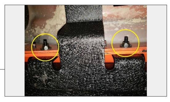
Align and fit the new Rubi Rail mounting studs through the vehicle pinch weld mounting holes. Tighten the Rubi Rail using the (4) M6 nuts and washers to the pinch welds.
